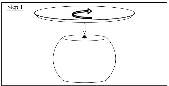
Place Base (B) onto a level surface with the top facing upwards. Align the threaded bolt at the top of Base (B) with the threaded hole on the underside of Top (A). Rotate the Top (A) clock-wise direction until it is fully tightened.
